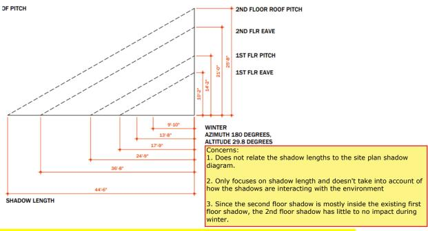
The second-floor roof pitch shadow above is mitigated below by only 16 inches (3%), from 44'6" to 43'2"
