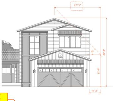
The design complies with the daylight plane. Also, the 2nd floor shifted back 4'1" in the new design.
